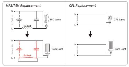
Note: Maxbrite Corn Light fixtures have an internal power supply that may  $\underline{not}$  be used with a dimmer  $\underline{not}$  becomes  $\underline{not}$  be used with  $\underline{not}$  becomes  $\underline{not}$  be used with  $\underline{not}$  becomes  $\underline{not}$
