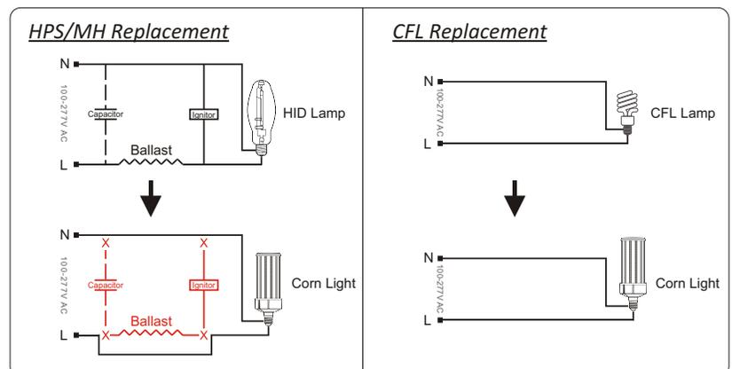
Note: Maxbrite Corn Light fixtures have an internal power supply that may not be used with a dimmer.
